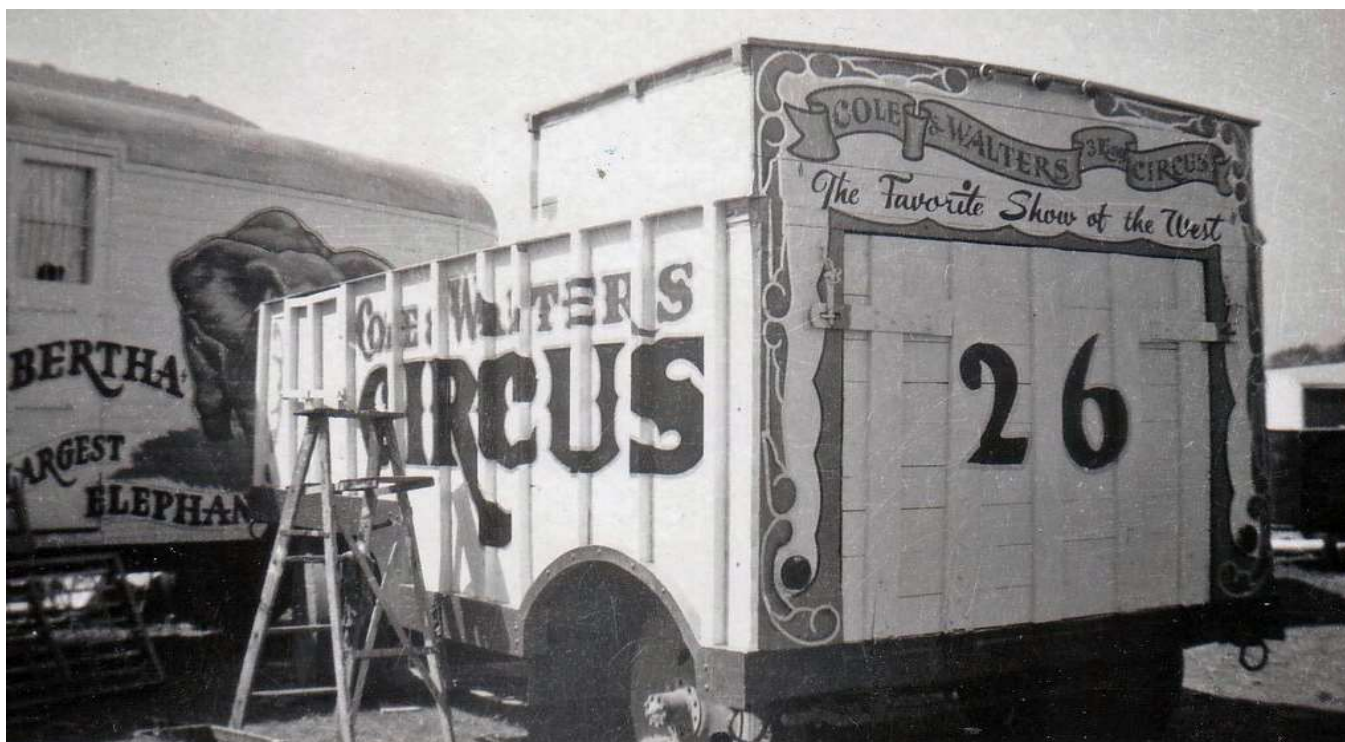
COLE and WALTERS CIRCUS Bandstand Wagon. This trailer No. 26 would be backed into the tent beside the back door. The tail gate folded down to become the bandstand. The "Favorite Show of the West" banner would be visible during the show above the band members' heads. Permanently installed inside the bandstand wagon was a Hammond Organ. The ring curbs and props were stored in the front section.
