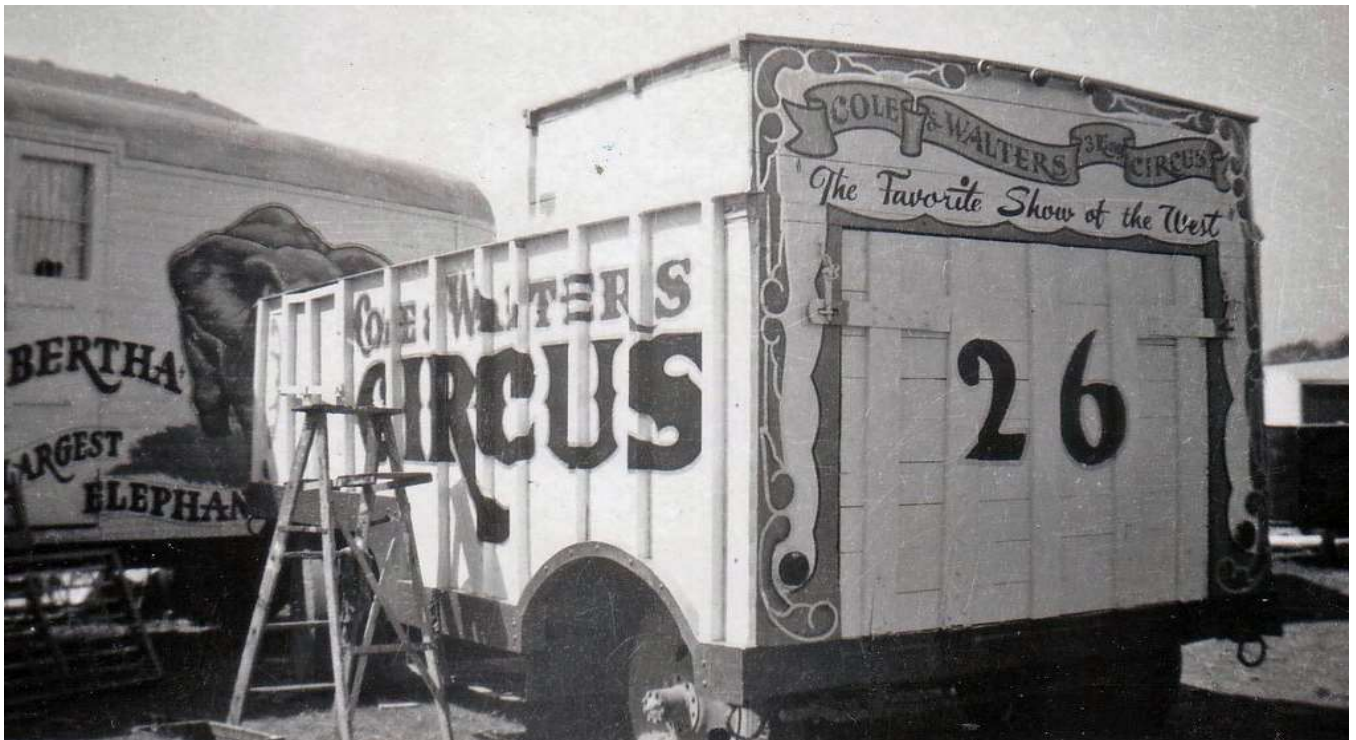
COLE and WALTERS CIRCUS Bandstand Wagon. This trailer No. 26 would be backed into the tent beside the back door. The tail gate folded down to become the bandstand. The "Favorite Show of the West" banner would be visible during the show above the band members heads. Permanently installed inside was a Hammond Organ. The ring curbs and props were stored in the front section.
